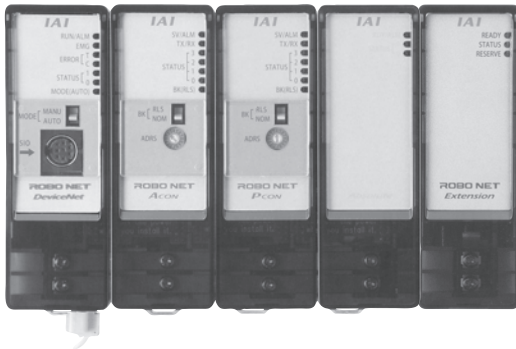
Gateway unit RACON unit RPCON unit Simple absolute R unit Expansion unit
